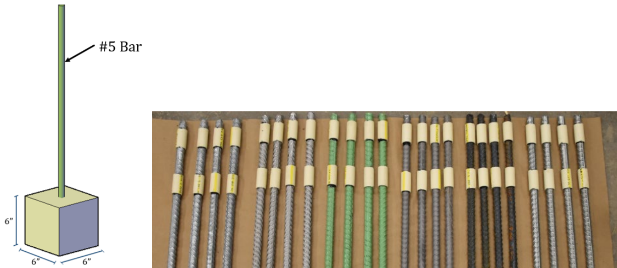
Figure 3 Pullout Specimen Details (Left) and Bar Types (Right)
