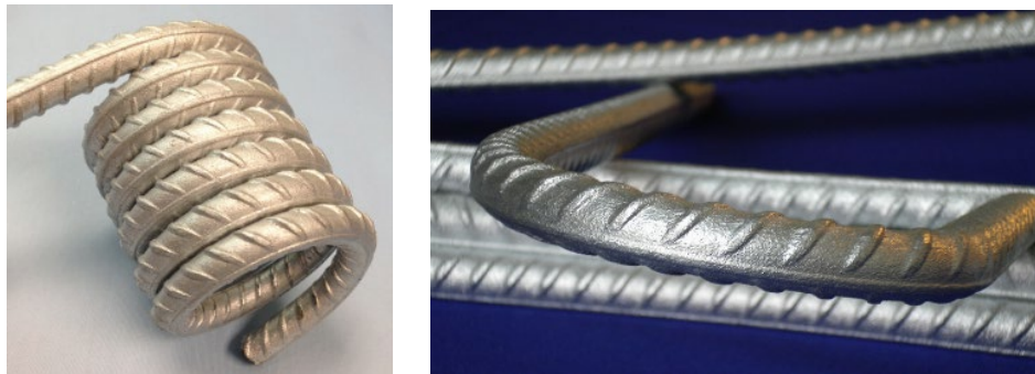
Figure 32 Bendability of GalvaBar
