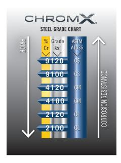
ChromX 9000 (ASTM A1035 CS Grade 100 or 120). This chromium alloy steel provides high corrosion protection for severe corrosive environments caused by seawater, aggressive soils and deicing salts. Designers can meet or exceed 100-year service life requirements called for on many infrastructure projects by specifying ChromX 9000.
